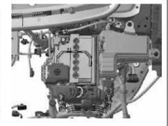
3. Battery in the engine compartment
