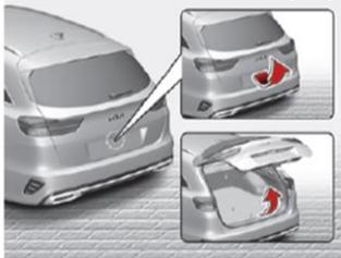
Unlock the tailgate with the smart key or the central lock button. Press the switch and pulling it up.
