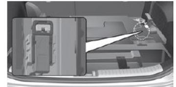
3. Pull up the yellow lever in the high voltage cut-off switch.
